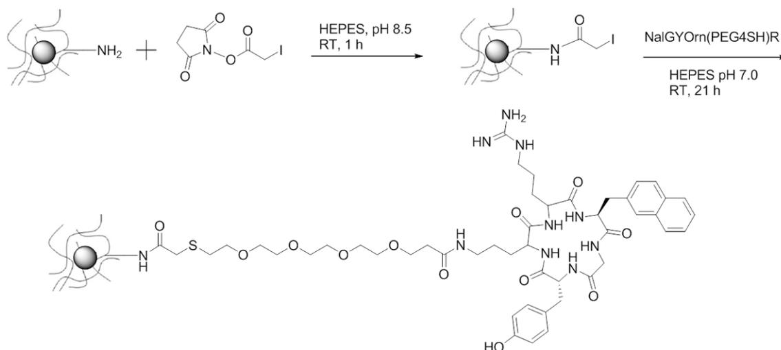
**Figure 4.** Scheme of NaIGYOrn(PEG<sub>4</sub>SH)R peptide conjugation to IONPs; Step 1: succinimide iodoacetate, amine functionalized IONPs, HEPES buffer (pH 8.5), room temperature, 1 hour; Step 2: NaIGYOrn(PEG<sub>4</sub>SH)R, SIA-functionalized IONPs, HEPES buffer (pH 7), room temperature, 21 hours; Purification by dialysis.
