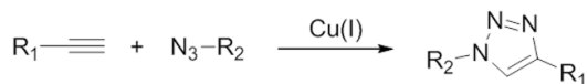
Figure 2. The Huisgen 1,3-dipolar cycloaddition is an extremely efficient click chemistry reaction, however the requirement of a toxic copper(I) catalyst to enhance the reaction rate has prevented its application in living systems.
